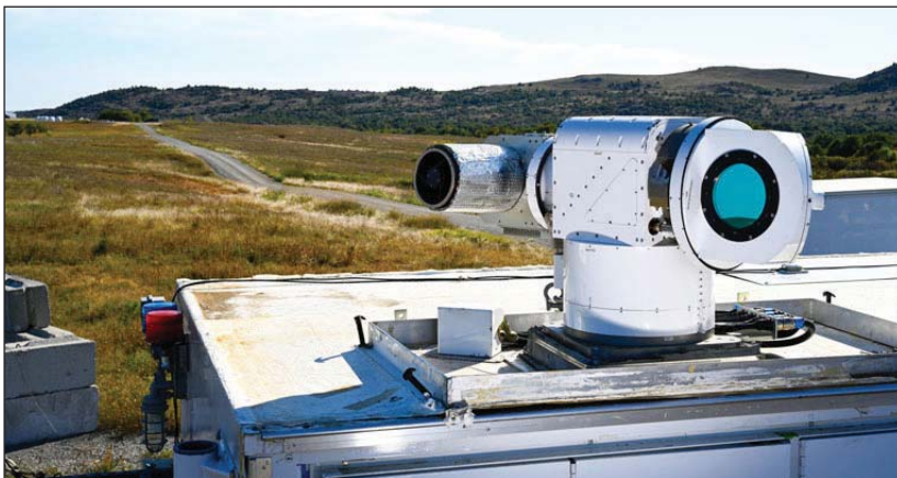
4. The ATHENA system is a HEL-based DEW designed as a defense against drones. (Courtesy of Lockheed Martin)
