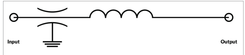
7. An "L" circuit adds an additional series of inductive elements to the "C" circuit.
